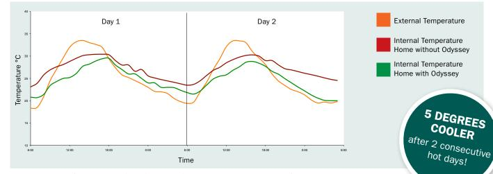
Measured temperature of a home in western Sydney fitted with two Odyssey prototype systems. Actual results for any home will depend on many variables including type of construction, location, shading, usage patterns etc.
